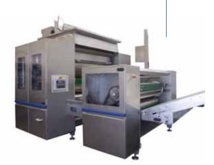
serves to produce dough bands for rotary-cut biscuits or for feeding a Frequency-controlled three-phase biscuit molding machine, respectively.
