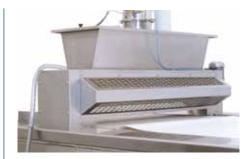
GAUGE ROLLER PAIR DUOMAT is used for calibrating pre-formed dough sheets to the desired thickness and for compacting and smoothening these dough sheets.
